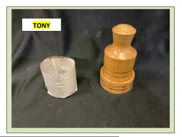
**TONY** and **TREV** made a top job of their paper pots maker. This little gadget is for growing plants from a single seed in a protected case then transferring the seedling together with its paper case to a plot in the garden. This approach minimizes/eliminates transplant shock as the tiny roots are not disturbed.
