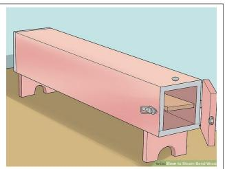
An easy-to-make steam box using wood. A length of PVC pipe would do the job just as well.
