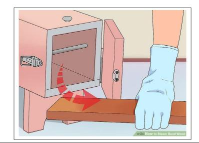
Remove the steamed wood with heat-resistant gloves when the time is up. Turn off the steam generator and carefully open the steam box with heat-resistant gloves. Remove the steamed piece of wood and begin the bending process as fast as possible before it loses its pliability.
