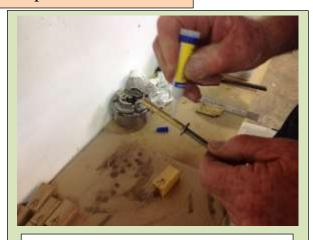
Holding the nail apply glue to the brass tube. (no glue on fingers eh)
