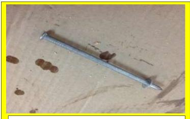
Fit a washer onto a six-inch nail. The diameter of the nail will fit inside a slimline brass tube.
