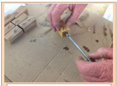
Now slide the gluey brass tube into the 7mm pre-drilled hole. (No mess Charlie eh)
