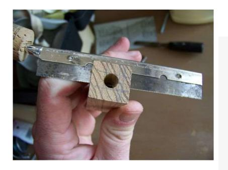
Start by using a **razor-sharp saw** to make a transverse cut approximately 25mm from the drilled end.
