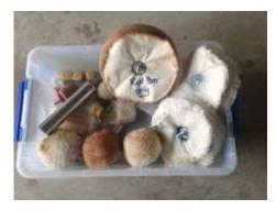
The **BEALL** buffing system uses a three stage approach. 1. **Red** Tripoli bar 2. **White** diamond bar. 3 **Yellow** carnauba wax bar.
