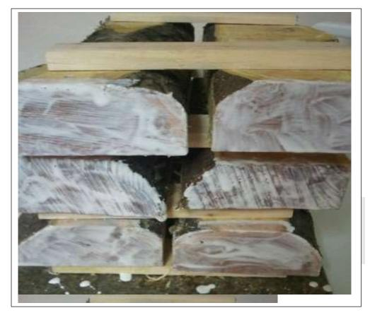
Here's a layered stack of timber slabs each of which has had a wax end-sealer generously applied.
