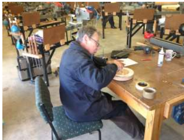
JAMES applies two coats of PVA glue to seal the wood. This is one method for preventing pesky bubbles emerging through curing resin mix.
