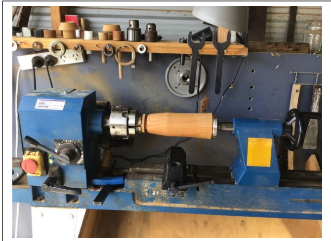
The engineer also made a tapered adapter to fit a live drive. This improvement will better enable goblets and vases to be held safely.
