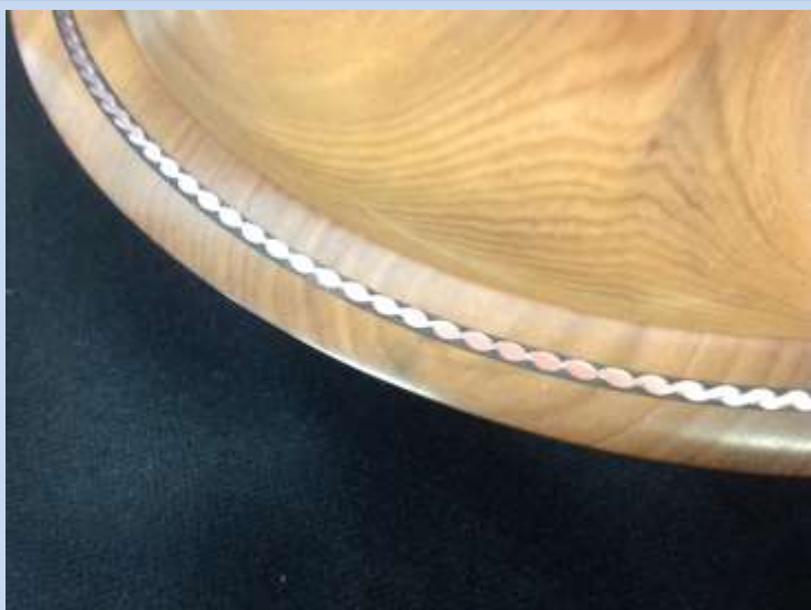
Here's a close-up shot of CAELAN's twisted copper wire set into a resin-filled narrow groove.
