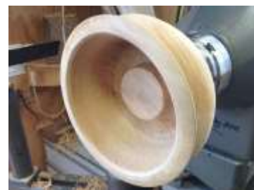
Thickish walls are OK. Now apply some wax coating.
