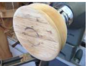
Mark out the “internal” spigot
