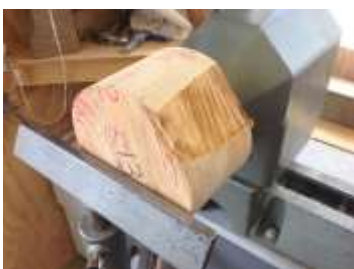
Mount onto the lathe
