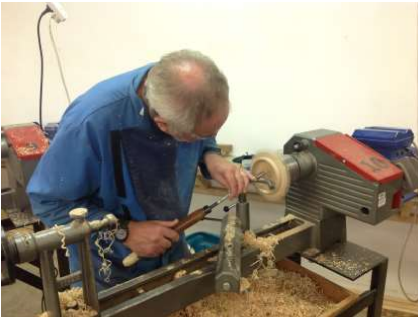
STEPHEN carefully removes the bottom of his well-designed bowl. It's a bit of a challenge to remove the spigot on the base but Stephen has plans to use a jam chuck and tailstock support to do the job.
