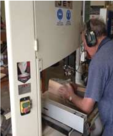
DAVE uses the large band saw to break down the NZ Oak to spindle size square sections. Now it's off to the drying racks.
