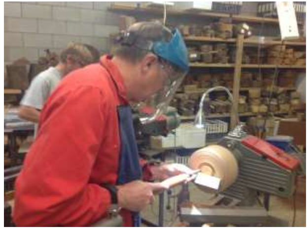
SPENCER forms a spigot on the base of his exceptional block of highly-figured rimu wood. This wood is outstandingly beautiful. (Hey Spencer, if the spigot finishes being too small you can switch to a 35mm chuck)
