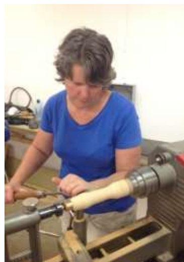
CHRISTINE is another new member who is also keen and quick to learn. A brass ferrule has been fitted and now the shaping of the knockout bar handle begins.
