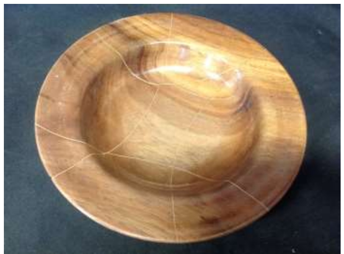
STEPHEN HAWLEY'S multi-veneered inset idea gives the bowl a spider-web appearance. Another notable feature is the high sheen finish. Cor! Well done!
