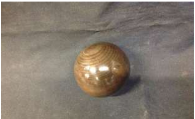
OSCAR used the Beall buffing system to get his high shine on his matai sphere.
