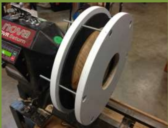
MALCOLM VAILE has made a "DOUGHNUT" chuck for holding turned bowls. This clever gadget enables the turner to work on the bowl base
