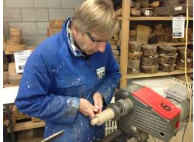
ANDRE` puts the finishing touches to his rewarewa wood pepper mill. The medullary rays, so prominent in this NZ native timber, were highlighted with the application of Liberon Finishing Oil.
