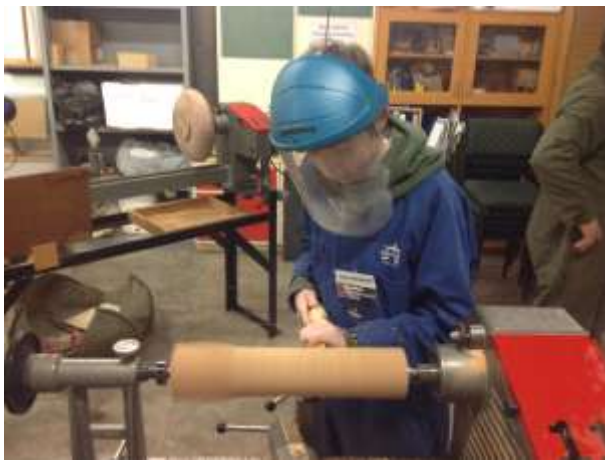
DYLAN sets to work turning a square section length into a cylinder.
