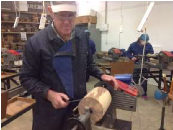
COLIN has been commissioned to turn an exacting mould blank to be used in a fiberglass lamp shade project. White maire was selected for this project as the wood always finishes well with a super-smooth surface. A slight hiccup occurred but was fixed by inserting a wooden plug to repair a hole made by bark inclusion.
