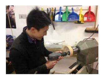
**DOMINIC** uses the power sander to remove any sign of stria and prepares the surface to finishing. In this case walnut oil was applied prior to the use of the EEE paste.
