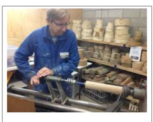
**ANDRE**` has found a new style of boring bit for drilling holes. This bit, in conjunction with an extender bar, should go a long way to solving the problem of long-hole drilling.
