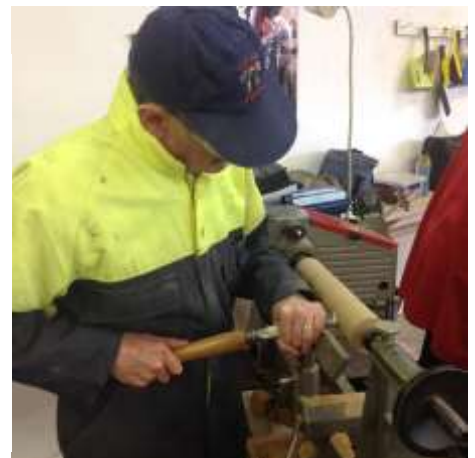
CHRIS prepares a cylinder of wood to be used for skew chisel practice.
