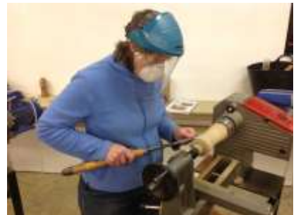
CHRISTINE has added the 40mm jamb chuck and starts the shaping of the pepper mill.
