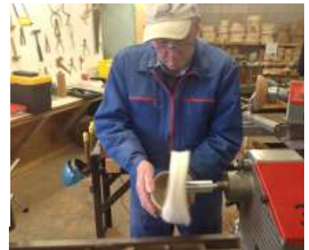
DES achieves a superb finish to his bowl project by using the BEALE buffing system
