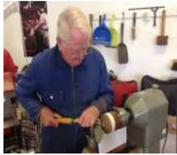
MALCOLM uses masking tape to align the grains while turning
