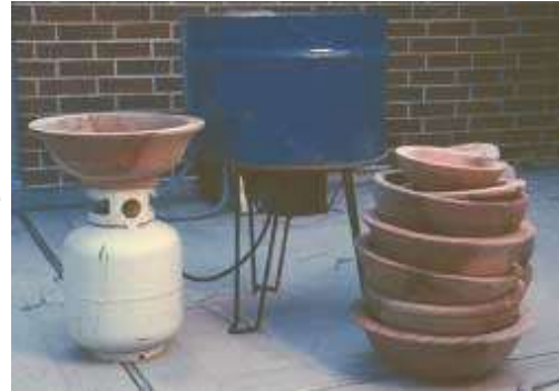
My setup for boiling green wood. Propane fired burner with a cut-down 55-gallon drum as the cooking pot.
