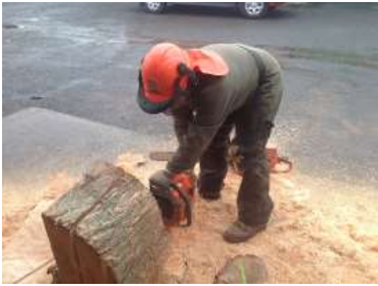
Muhannad chainsaws the logs into slabs
