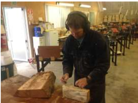
Paul checks each slab and marks out the "rounds"
