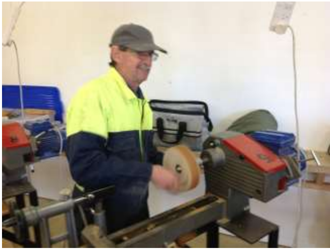
CHRIS put the finishing touches to his tool handle using the Beale buffing system.
