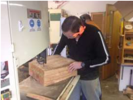
Spencer uses the band saw to cut out the "rounds":
