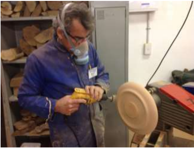
Above: ROBERT power sands the underneath side of his platter project that will have colour added.
