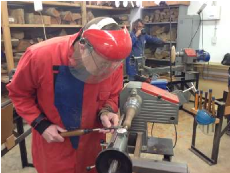
SPENCER makes a handle for his scraper tool. The ferrule is carefully fitted prior to final shaping for custom fitting of his hand.
