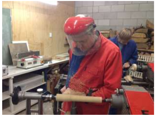
Above: SPENCER turns a handle for his scraping tool using ideal ash wood.
