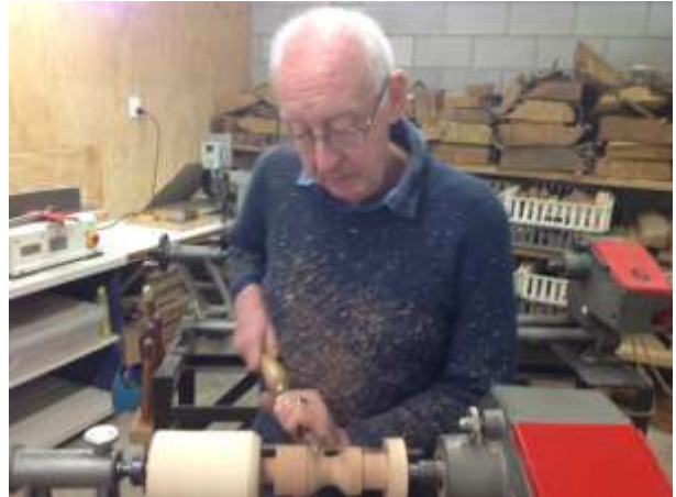
MALCOLM prepares to drill a hole to take the tang of an old steel file which will eventually be turned into a woodturning scraping tool.
