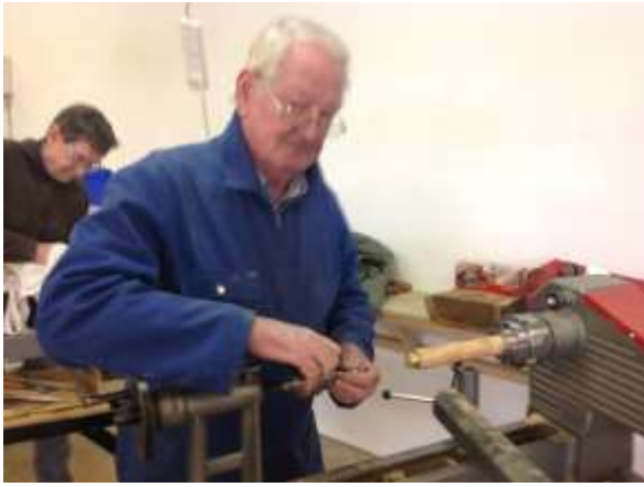
RIGHT: Spindle turning DAVID turns the head of his pepper mill. A jamb chuck assists with the correct lining up of the mill parts.
