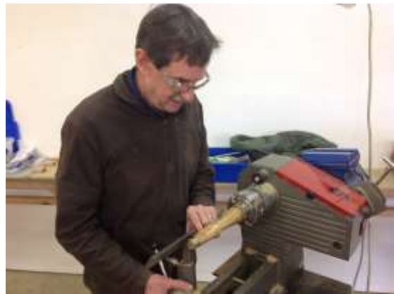
RIGHT: CHRIS very quickly fashioned a ferruled handle for his scraper then fitted the tang using two-pot epoxy resin. A second scraper was commenced soon after.
