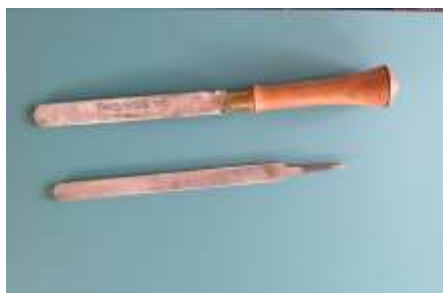
Two old steel files destined to become useful round-nose scrapers
