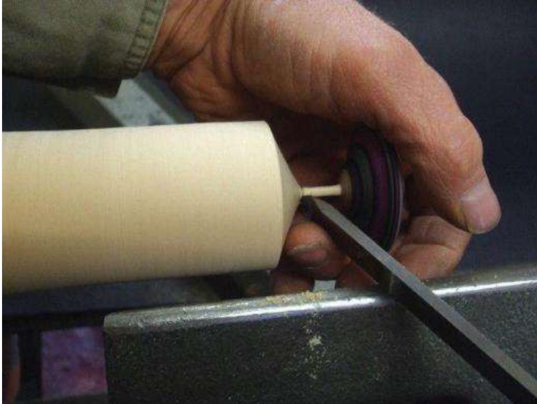
Soft Landing – With your hand loosely around the spin top, part it off.
