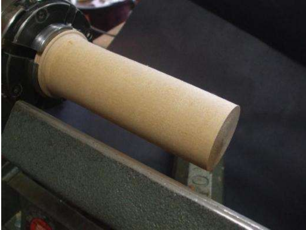
Large Dowel – The first step is to turn a cylinder just over 2" in diameter. Each top is cut from the end of this cylinder. Use a roughing gouge for this job.
