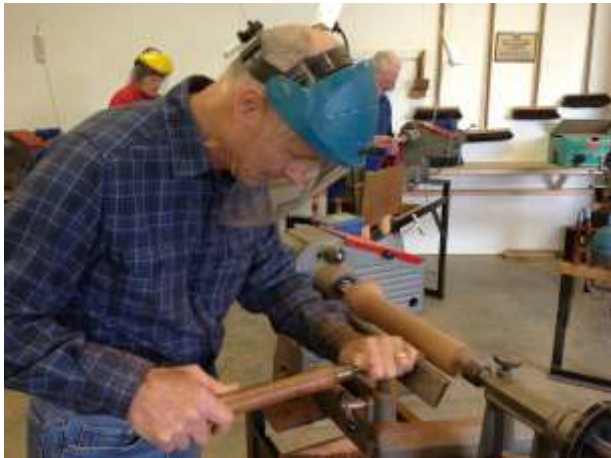
Above picture: DAVID turns the leg for one of a pair of lamp stands. The big challenge next is to drill a long hole through the leg shaft to take the electric cord.
