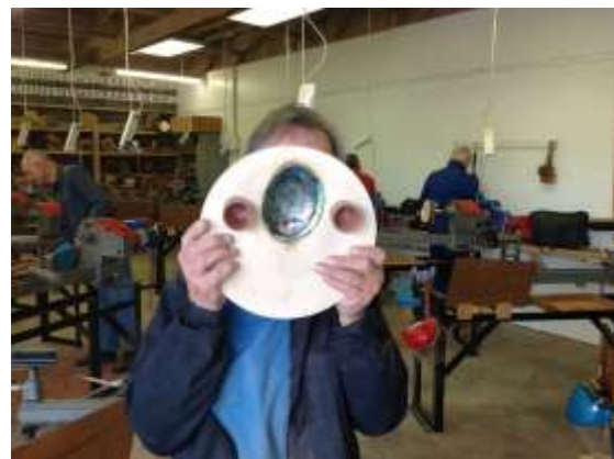
Above two pictures: JAMES is turning one of two small condiment pots for his paua platter. The paua shell is set in a carved-out cavity and rests on a bed of epoxy resin that holds it firmly in place.
