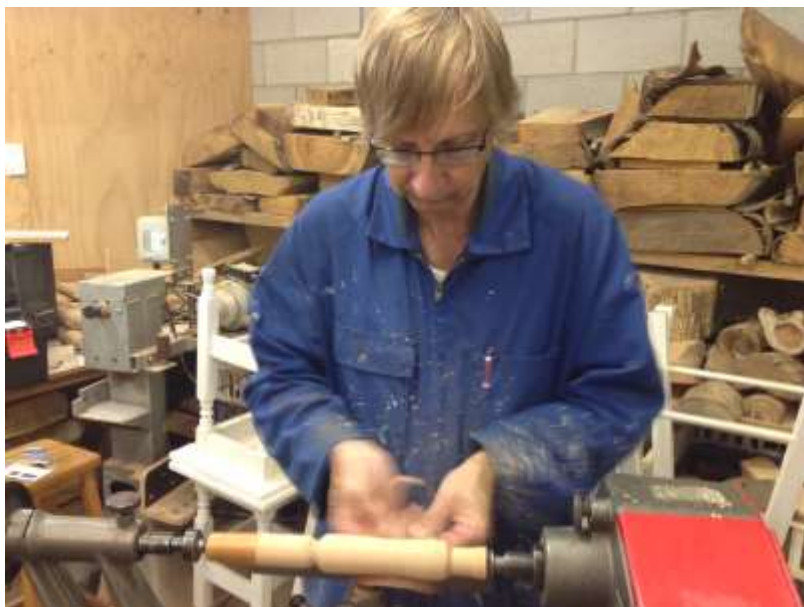
ANDRE` adds the finishing touches to his wooden tool handle. Later he fitted a 10mm stainless steel rod and brass ferrule to the handle and Hey Presto ! – knockout bar completed - all done in one session. Wow!
