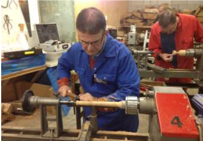
Above: Concentration and determination here! MIKE prepares a cylinder of black maire wood to make another paper knife.
