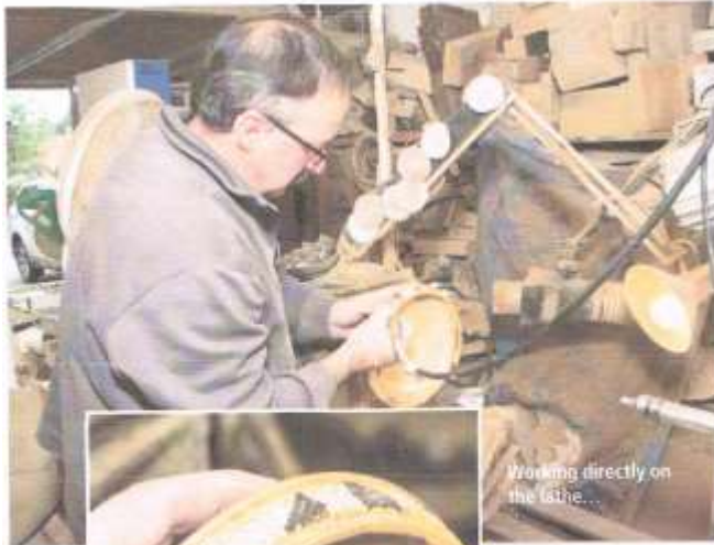
Jig mounted to allow the Dremel to be used with a bowl chucked in the lathe.
