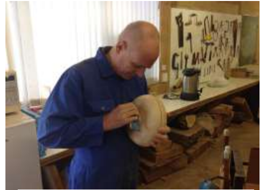
DAVID has to figure out how to refit the faceplate so he can remount his bowl to adjust the size of the spigot to fit a 35mm power jaw.
