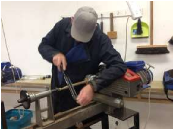
Colin uses a special scraper to flatten the surfaces of the knife blade.
