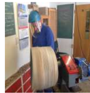
How to wet-turn a bowl out of a mammoth block of Norfolk Pine. Grant Taylor took on this mighty challenge then skillfully figured out ways of getting it balanced and carefully shaped. A special challenge – a special achievement! El Biggo!
