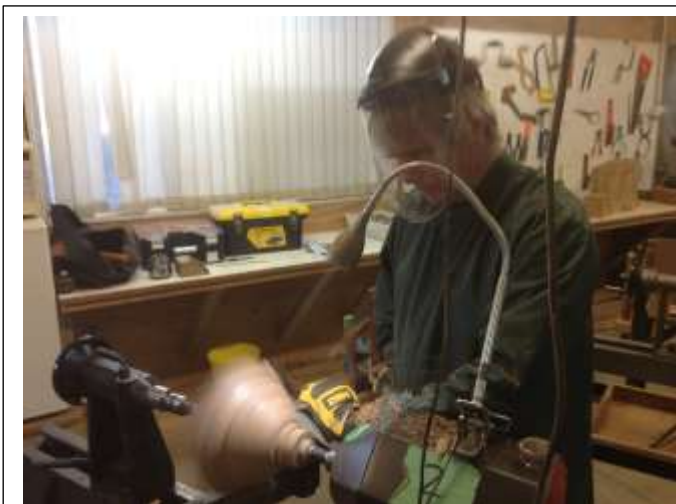
GARY works away at shaping the all-important spigot (Don't forget the "Wall" for the jaw faces).
