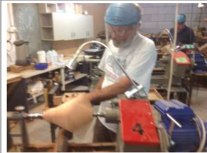
DAVID made good progress with the initial cut putting the spigot end at the tailstock
